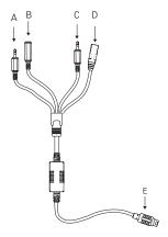
Figure 4. AccuMic VC connector cable
